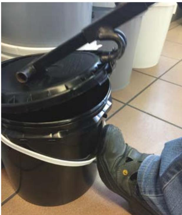
This opening device can be used with all of our product ranges that are fitted with eyelets.
