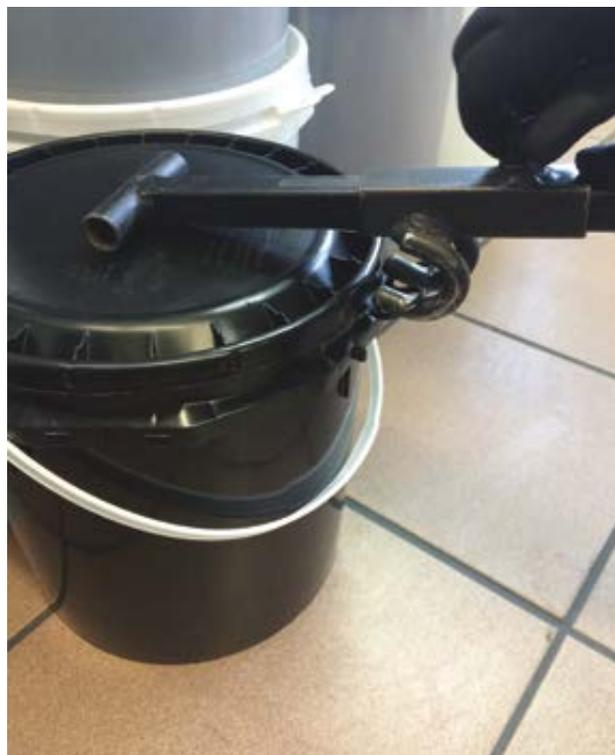
2. Lift the bar towards you, the lever mechanism will allow the lid to open easily.
