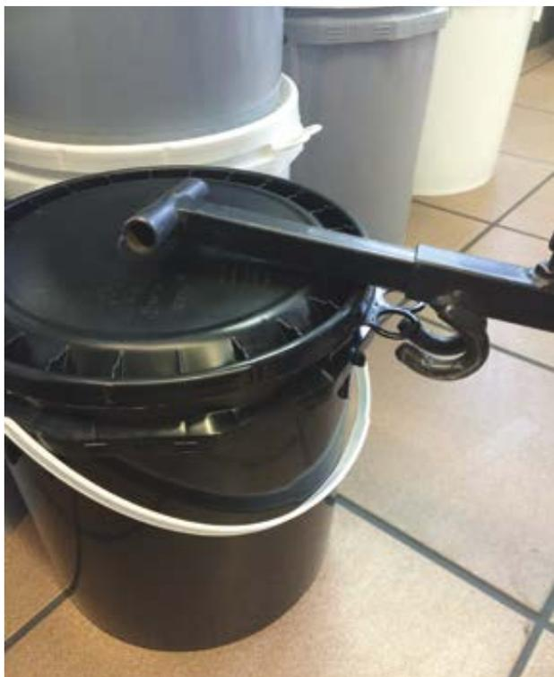
1. Place the two hooks of the metallic bar into the opening eyelets.
